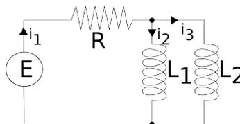
Solve the system if  $R = 5 \Omega, L_1 = 0.01 \text{ h}, L_2 = 0.0125 \text{ h}, E = 100 \text{ V}, i_2(0) = 0$  and  $i_3(0) = 0.$  Also determine the current  $i_1(t).$
